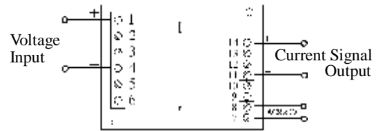
Fig. 3.4.8 CE-P02, CE-Q02 Current Output, Case style SK
