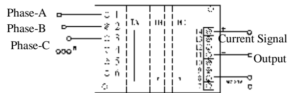
Fig. 3.4.12 CE-P41, CE-Q41 Current Output, Case style SK
